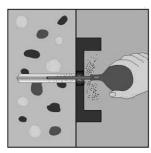
Removal of drill dust e.g. blowing
