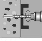
Installation e.g. by hand or with impact screw driver
