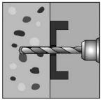
Drilling Drill diameter  $d_0$  and drilling depth  $h_1$  have to be met
